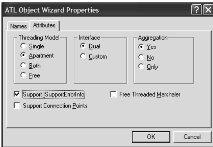
Figure 8-25. Supporting ISupportErrorInfo using ATL
