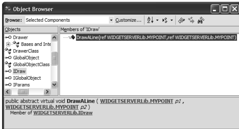
Figure 8-7. Mapping COM structures of System.ValueTypes
